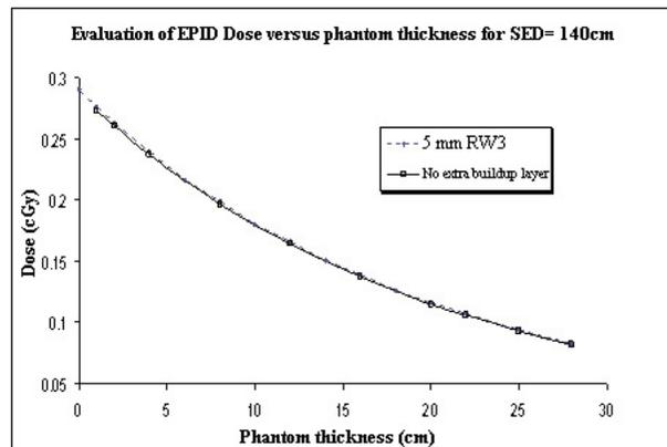
**Figure 2.** The variation of transmitted dose with the increase of a homogeneous phantom thickness on the central axis using 6 MV photon energy for a 10×10 cm<sup>2</sup> field size, at SED=140 cm and dose rate 300 MU/min. All EPID images were acquired in fast read-out and full resolution mode. Each point is the average of two consecutive measurements.
