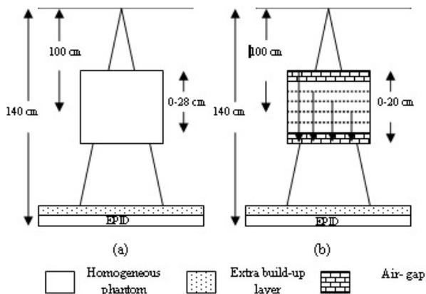
**Figure 1.** Schematic view of the measurement set-up to evaluate the EPID response versus the phantom thickness. (a) Experimental set-up for EPID response for various thicknesses of homogeneous phantom. (b) Experimental set-up for EPID response for various positions of 2 cm air gap inhomogeneity.
