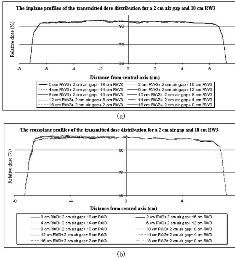
**Figure 7.** (a) Inplane profiles of the transmitted dose map using a SLIC-EPID with various position of 2 cm air gap within the 18 cm RW3 phantom. (b) Crossplane profiles of the transmitted dose map using a SLIC-EPID with various position of 2 cm air gap within the 18 cm RW3 phantom. All data are the average of two consecutive EPID images acquired with 6 MV photon energy beam, 300 MU/min, 10×10 cm<sup>2</sup> field size and SED= 140 cm.
