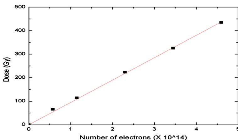
Figure 1. Dose calibration curve for Microtron Accelerator.
