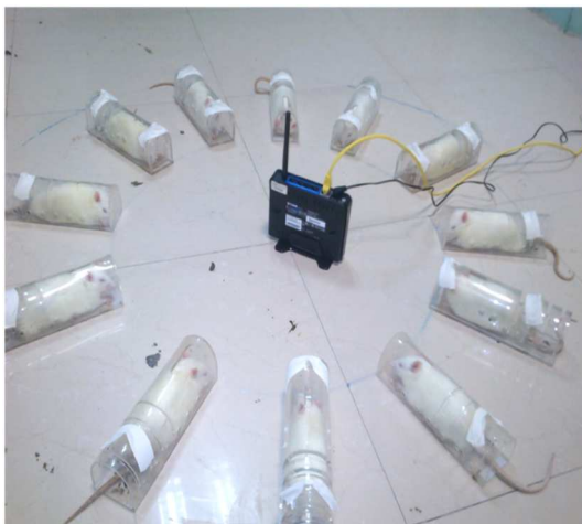
Figure 1. Irradiation geometry. Rats were placed in Plexiglas restrainers and exposed/sham exposed to Wi-Fi radiation at a distance of 30 cm or 60 cm from the router.
