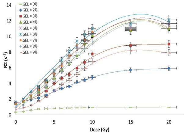
Figure 6. Transverse relaxation rate (R2) as a function of absorbed dose (D) for MAGAT gel dosimeter composed of 9% MAA and at various concentrations of gelatin.
