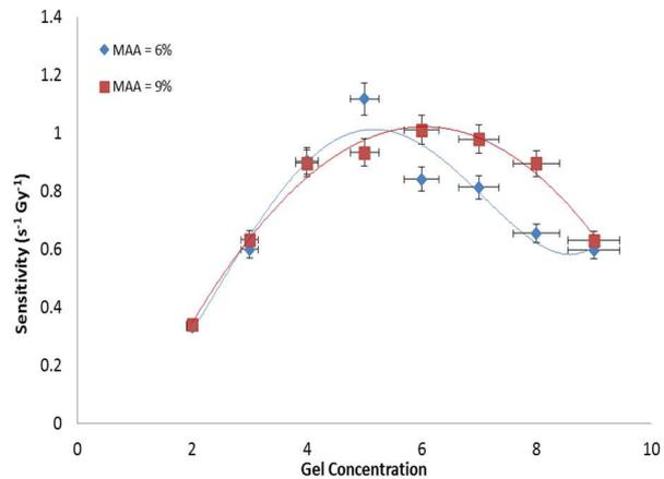
Figure 8. The sensitivity of MAGAT gel dosimeter as a function of gelatin concentration at different MAA.
