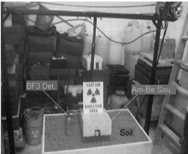
Figure 5. Photograph of landmine detection set-up.
