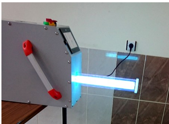
Figure 1. UV-C ultraviolet generator used in the study.
