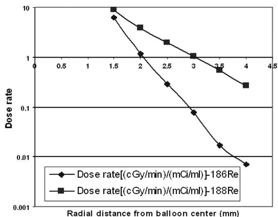
**Figure 4.** Depth dose rate distribution in [(cGy/min)/(mCi/ml)] in  $z=0$  plane was calculated for  $^{188}\text{Re}$  and  $^{186}\text{Re}$  solution that balloon had the diameter of 3mm and length of 20mm.
