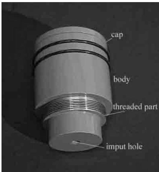
Figure 2. Stereotactic collimator used for limiting radiation fields to desired dimensions.
