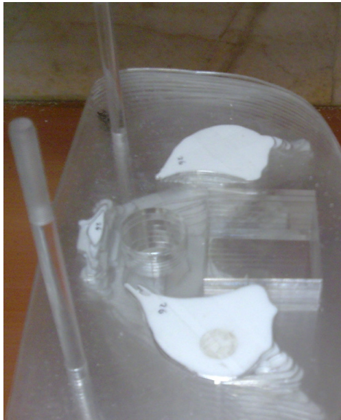
Figure 2. The opened slice anthropomorphic phantom.
