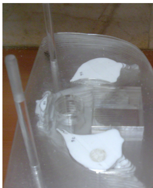
Figure 2. The opened slice anthropomorphic phantom.
