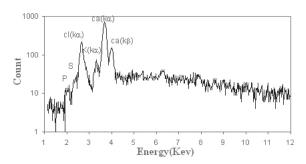
Figure 1. Typical spectra for shell of pigment stones (With a 175 µm Mylar filter).
