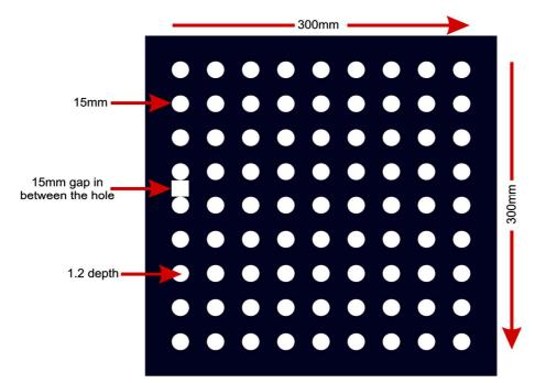
Figure 3. Custom build TLD holder plate made out of PMMA.
