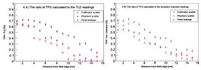
Figure 4. Different components contribution for out-of-field dose for an open field of  $10 \times 10 \text{ cm}^2$  at 5 cm depth.
