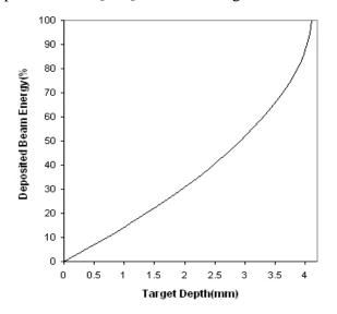
**Figure 6.** Calculated estimate of energy deposited by the beam as percentage of total for 18MeV protons incident to the <sup>18</sup>O-water target.
