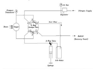
**Figure 4.** Schematic representation of the unit for remotely filling the <sup>18</sup>O-enriched water target at the NRCAM cyclotron unit.
