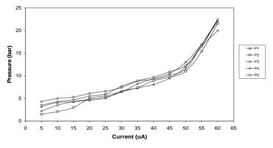
Figure 5. Pressure in the target chamber Vs. beam current (18MeV protons).
