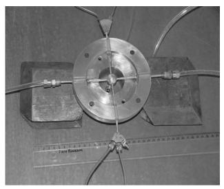
**Figure 2.** Picture of the spherical gold target with brass holder and tubes for cooling and loading the target.
