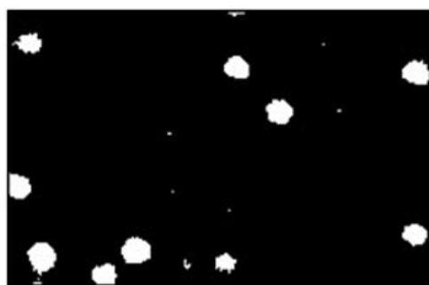
Figure 2. The tracks of alpha particles formed on LR-115 plastic track detector
