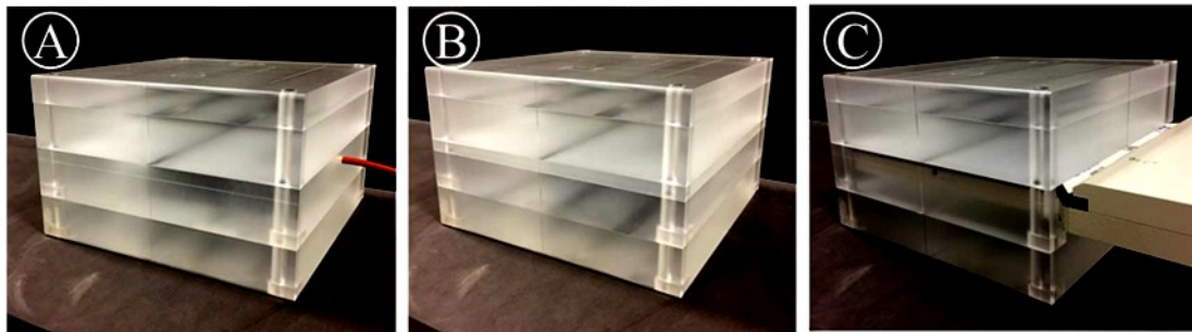
Figure 1. A multi-purpose phantom using (A) the ionization chamber, (B) the EBT3 film, and (C) the MapCHECK system.
