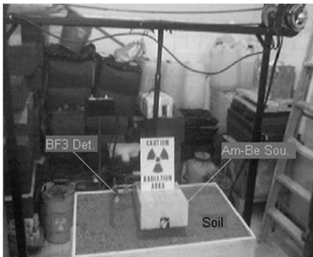
Figure 5. Photograph of landmine detection set-up.
