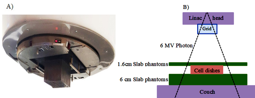
Figure 2. A) The clinical Grid block mounted on the Varian 2100C linear accelerator (Linac); B) Schematic view of the irradiation setup.
