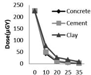
**Figure 4.** Attenuation of Cs-137 gamma rays as a function of thickness through different shield materials.
