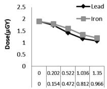
**Figure 1.** Attenuation of Co-60 gamma rays as a function of thickness through different shield materials.
