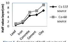
Figure 5. Comparison of half value layer of different Materials using different γ-rays sources.
