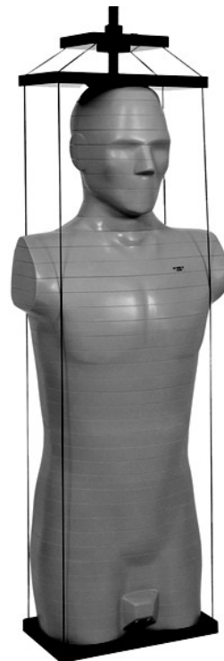
Figure 2. TLD locations and the number of TLD used are sorted by the slice number of the RANDO phantom in order to measure the delivered dose for each technique. FJ refers to Field Junction.
