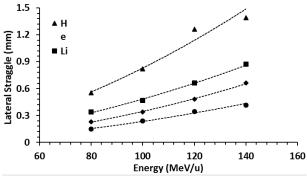
Figure 3. Lateral straggle for 80-140 MeV/u heavy ion beams.
