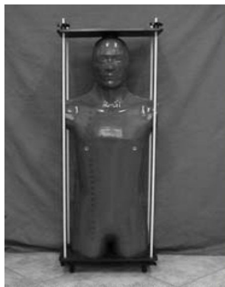
Figure 1. Alderson Rando phantom.
