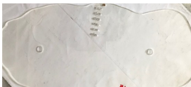
Figure 2. Slice number of 16 has several holes with a diameter of about 5.0 mm for introducing a dosimeter such as a TLD in different depths. The holes were numbered to provide an accurate dose estimate for each measurement.
