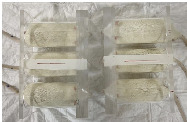
Figure 2. The image of rats that will be subjected to whole brain irradiation in plexiglass tubes designed for immobilization. Rats anesthetized in the prone position underwent skull irradiation with a single dose of 30 Gy at a dose rate of 1 Gy/min.
