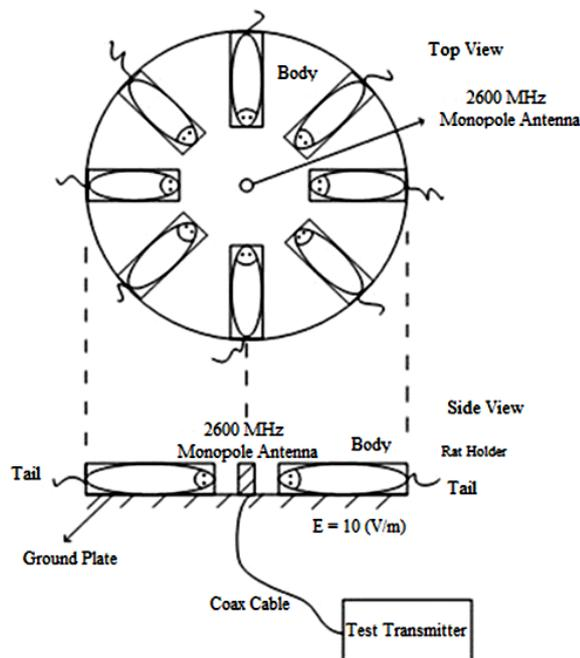
Figure 1. Schematic view of the 2600 MHz exposure setup.
