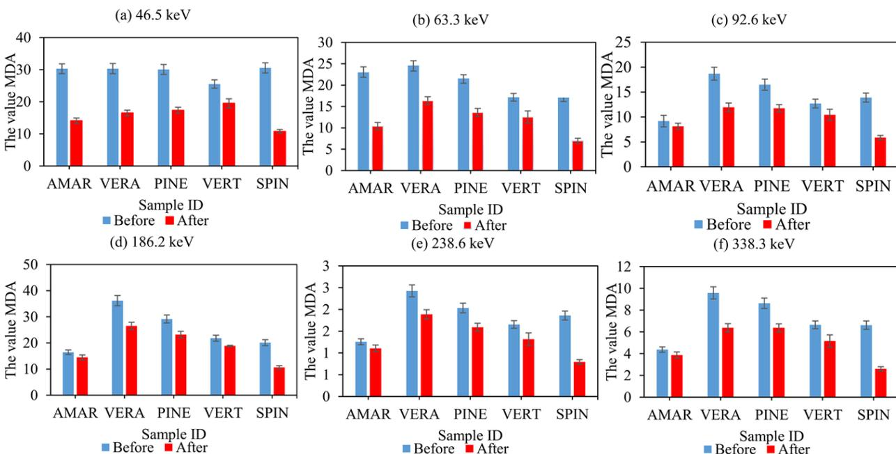
Figure 6. Comparison of the MDA values before and after K-separation for different gamma energies impacted by the <sup>40</sup>K Compton region: (a) 46.5 keV, (b) 63.3 keV, (c) 92.6 keV, (d) 186.2 keV, (e) 238.6 keV, and (f) 338.3 keV.
