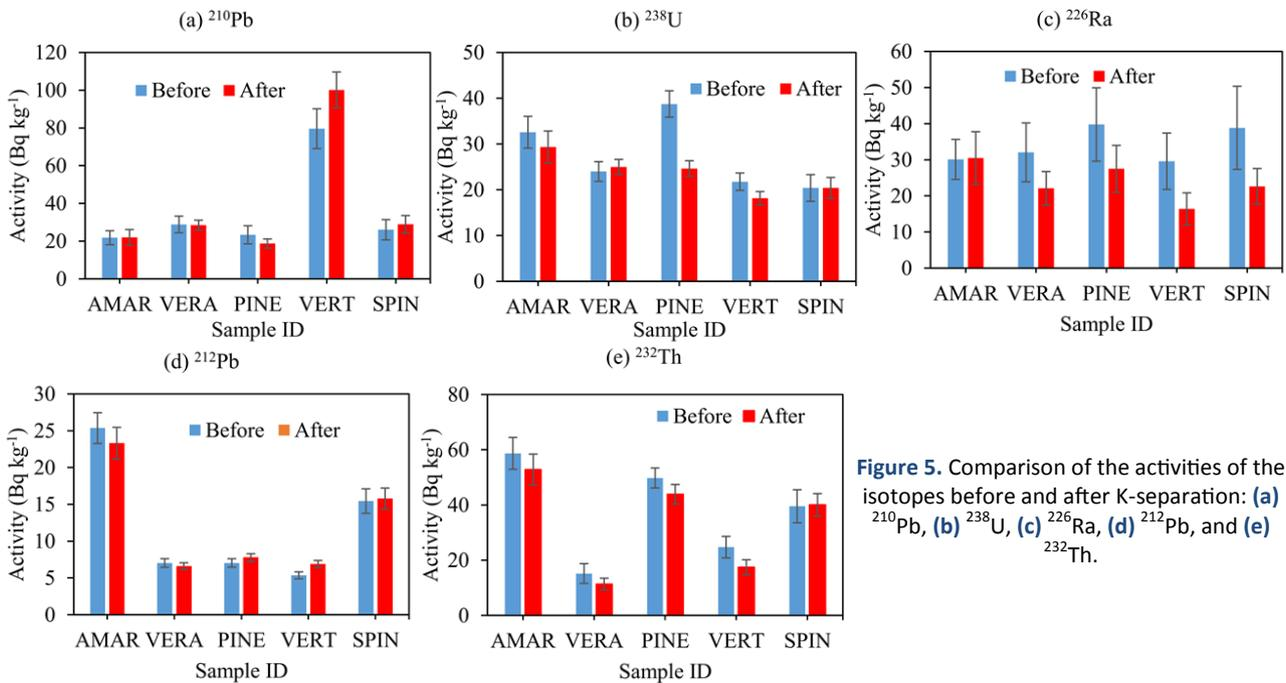
Figure 5. Comparison of the activities of the isotopes before and after K-separation: (a) <sup>210</sup>Pb, (b) <sup>238</sup>U, (c) <sup>226</sup>Ra, (d) <sup>212</sup>Pb, and (e) <sup>232</sup>Th.
