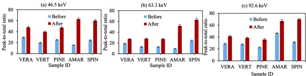
Figure 4. Comparison of the peak-to-total ratios of the low-energy peaks before and after K-separation: (a) 46.5 keV of <sup>210</sup>Pb, (b) 63,3 keV of <sup>232</sup>Th, and (c) 92.6 keV of <sup>232</sup>Th.
