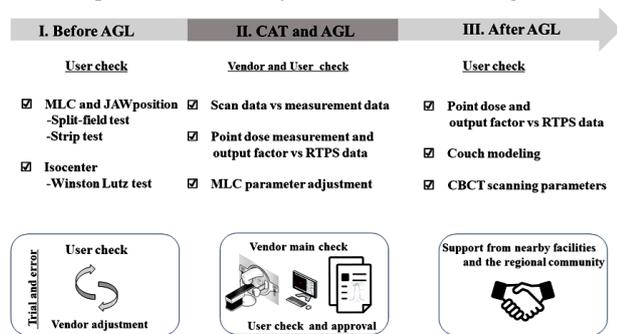
**Figure 1.** Study flow chart. AGL, accelerated go live; CAT, commissioning and acceptance test; MLC, multileaf collimator; RTPS, radiation treatment planning system; CBCT, cone beam computed tomography.
