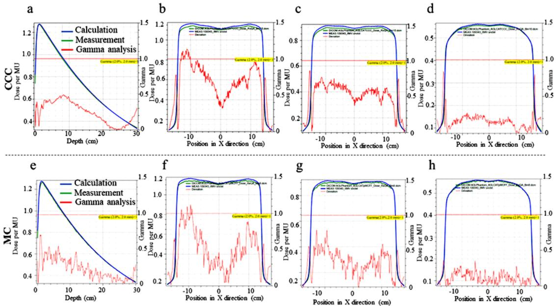
**Figure 2.** AGL result of the PDD and OCR for 30×30 cm<sup>2</sup> irradiation field size of 6 MV, (a) CCC, PDD, (b) CCC, OCR for depth of 5 cm, (c) CCC, OCR for depth of 10 cm, (d) CCC, OCR for depth of 15 cm, (e) MC, PDD, (f) MC, OCR for depth of 5 cm, (g) MC, OCR for depth of 10 cm, and (h) MC, OCR for depth of 15 cm.
