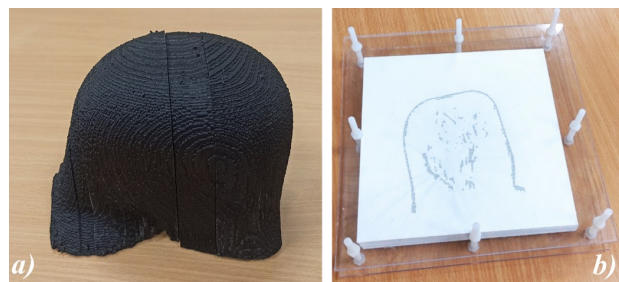
Figure 3. Phantoms used in the study: (a) FDM phantom, (b) Paper phantom. The digital source of these phantoms was the same.
