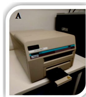
Figure 2. TLD readers: Harshaw 3500 manual reader (Thermo Fisher Scientific, USA) (A), and PCL3 automatic reader (Fimel, France, Europe) (B).
