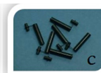
Figure 3. TLD -100 in the form of powder (A), capsule' (B), and black plastic capsules (C).
