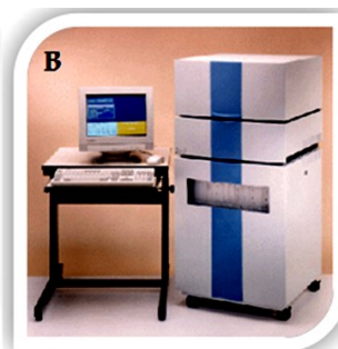
Figure 2. TLD readers: Harshaw 3500 manual reader (Thermo Fisher Scientific, USA) (A), and PCL3 automatic reader (Fimel, France, Europe) (B).
