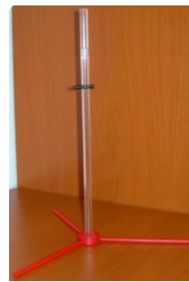
Figure 11. The IAEA standard holder where the dosimeter is placed during irradiation at the participating center.
