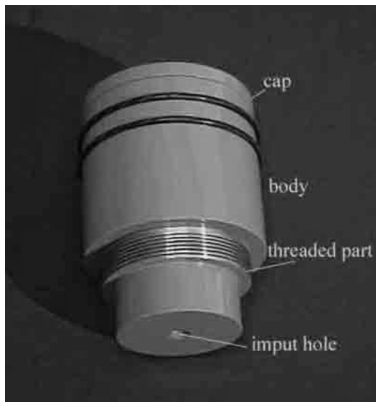
Figure 2. Stereotactic collimator used for limiting radiation fields to desired dimensions.
