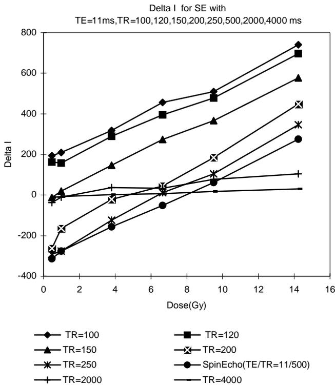
**Figure 2.** Signal intensity versus dose for TE=11ms and TRs=100,120,150,200,250,2000 and 4000ms in SE technique.
