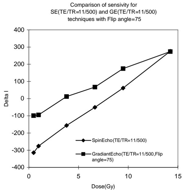
**Figure 3.**  $\Delta I$  profiles for dose range of 0.47 to 14.23 Gy, 1) SE technique with TE=11,TR=500 and 2) GRE technique with TE=11,TR=500 and flip angle 75. The sensitivity in (SE) is  $39.9 \text{ Gy}^{-1}$  while for (GRE) is  $26.9 \text{ Gy}^{-1}$ .
