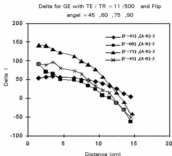
**Figure 5.** Curves obtained with GRE technique for  $TE=11ms$ ,  $TR=500ms$  with flip angles of  $45^\circ$ ,  $60^\circ$ ,  $75^\circ$ , and  $90^\circ$ . phantoms were Plexiglas irradiated to a certain dose.
