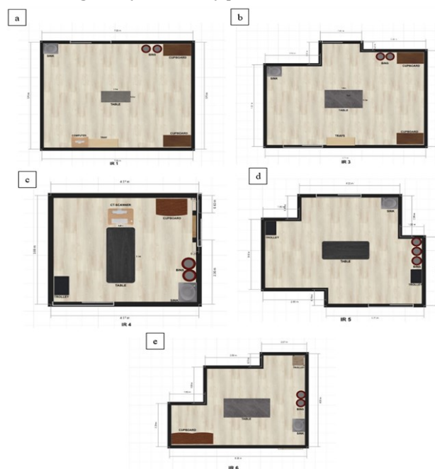
Figure 1. Geometries of angiography rooms for simulation (a) IR1, (b) IR3, (c) IR4, (d) IR5, (e) IR6. The geometries represent different interventional radiology suites within the clinical setting, each with unique room dimensions. These room geometries were modelled based on actual floor plans and equipment layouts to accurately reflect clinical practice and ensure realistic dose estimation using the Monte Carlo GATE simulation framework. (IR 1 (5.75 x 7.00) m, IR 3 (4.55 x 7.70) m, IR 4 (3.89 x 4.57) m, IR 5 (3.43 x 5.76) m, IR 6 (4.22 x 4.65) m measurement).
