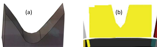
Figure 7. (a) The graphical Shape of body bowtie filter of PET/CT Biograph 6 (present study). (b) Body bowtie filter shape of Siemens Biograph 16 true point PET/CT that are estimated by using the Accu-Gold kit Radcal (Radcal Corporation, Monrovia, CA) with AGMS-Dsensorex.
