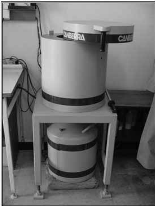
Figure 1. Gamma spectrometry detector shield.
