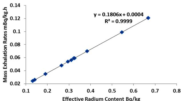
Figure 3. Linear relationship between mass exhalation rate for radon and effective radium content.
