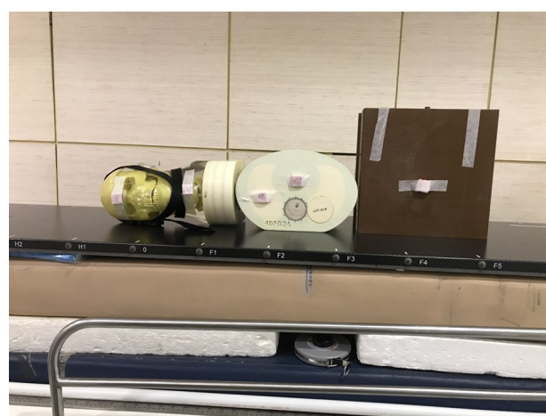
Figure 3. TBI phantom for mid-plane dosimetry.
