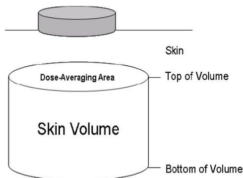
Figure 1. Schematic of the volume average dose model.
