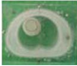
Figure 1. Transverse section of the heart and chest phantom composed of four cylinders, 15 cm long, which represent soft tissue of body contour, lungs, heart wall, and internal blood of the heart.
