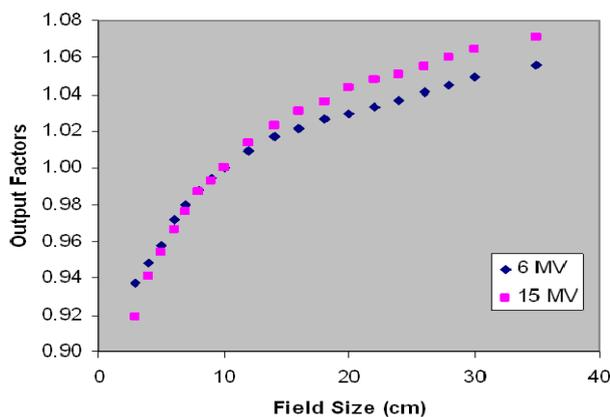
**Figure 2.** Variations of output factors with field size measured with compact cylindrical ionization chamber and acrylic build up cap.
