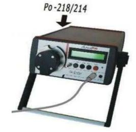
Figure 1. Typical alpha progeny meter (Saphymo GmbH).
