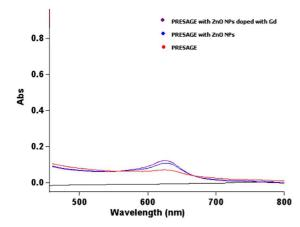
**Figure 3.** The absorption spectrum of various compositions of PRESAGE over visible wavelengths.
