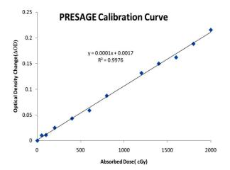
Figure 4. Calibration curve of PRESAGE.
