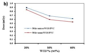
Figure 5. The dose measured after the micro and nano- structured shields with 1.1 cm thickness as a function of the weight percentage (wt %) of WO<sub>3</sub> for (a) 40 kV and (b) 50 Kv X-ray beam.
