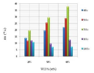
Figure 4. percentage difference between the mass attenuation coefficients  $(m/\rho)$  of nano and micro-structured samples, (m), as function of  $WO_3$  weight percentage for different X-ray voltages.
