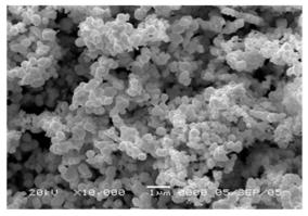
Figure 1. The SEM image of the nano-WO3 powder.
