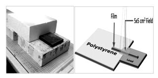
Figure 1. Heterogeneous phantom setup to test dosimetry properties in enhanced scatter and beam filtering conditions.
