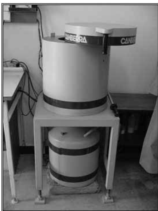
Figure 1. Gamma spectrometry detector shield.
