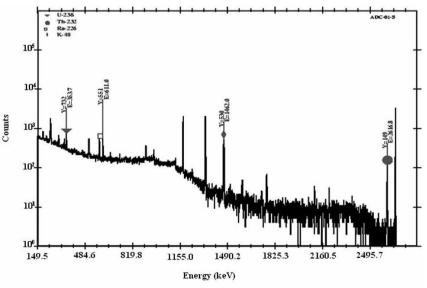
Figure 3. The gamma ray spectrum for soil sample.
