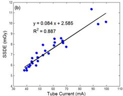
Figure 8. The relationships between average tube current and SSDE for (a) abdomen and (b) thorax.
