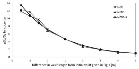
**Figure 8.** Comparison of MC simulation results and newly suggested formula for scenarios **a)**, **b)** and **c)** with and without steel barrier from figure 2. CORR presents the new empirical formula and MCNP computational results.
