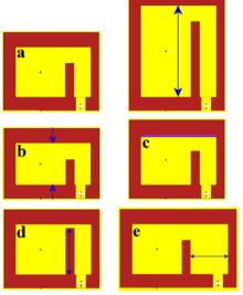
Figure 2. Ground plans for all simulated scenarios. Air is represented in yellow, concrete in dark red and additional steel barrier in purple: Blue arrows show direction of dimension change. a) Initial structure (maximum elongation on the right side), b) maximum contraction, c) addition of steel, d) maximum elongation of steel wall and e) maximum elongation of maze width.
