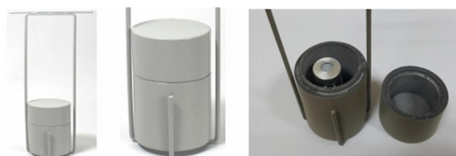
Figure 2. Moly-Shield used for the radionuclide purity measurement.
