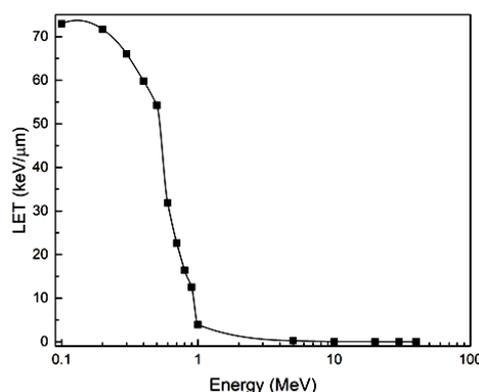
Figure 2. LET for different proton energy levels.
