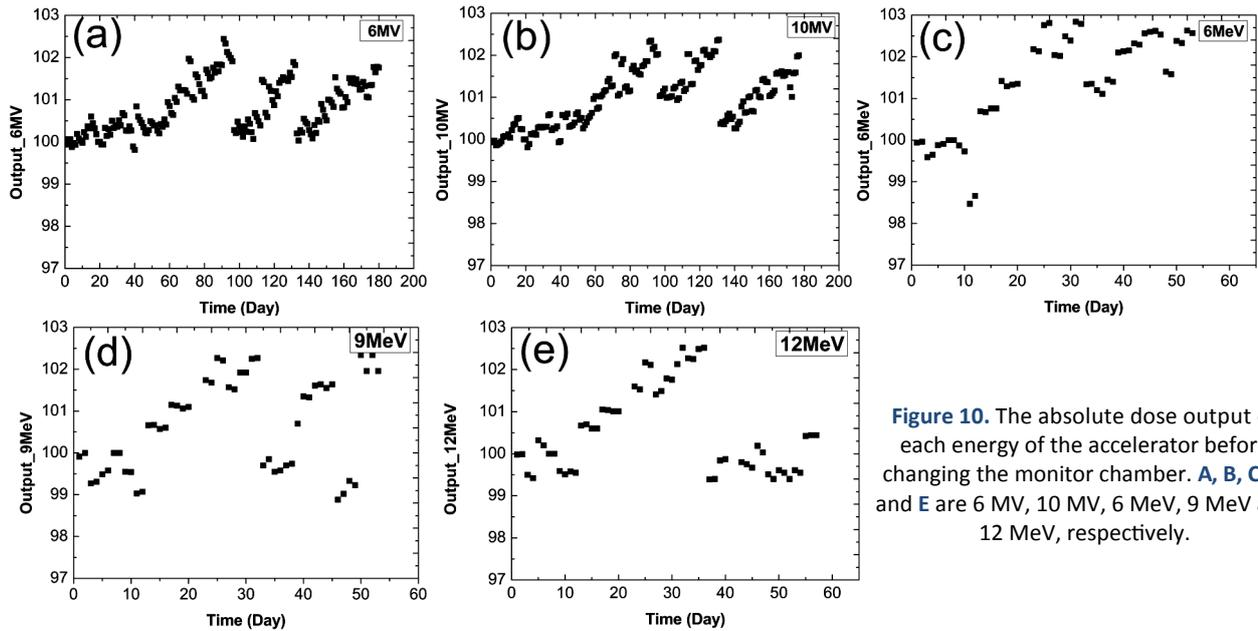
Figure 10. The absolute dose output of each energy of the accelerator before changing the monitor chamber. A, B, C, D and E are 6 MV, 10 MV, 6 MeV, 9 MeV and 12 MeV, respectively.
