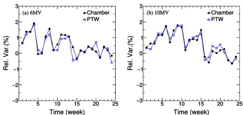
Figure 3. Variations in output constancy from baseline values for QUICKCHECK<sup>webline</sup> and the Farmer ionization chamber measuring a Varian ix (Sn: 6324) linear accelerator at an energy of (A) 6 MV and (B) 9 MV.
