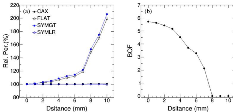
Figure 7. The output of PTW QUICKCHECKweblin in the gun-target direction.
