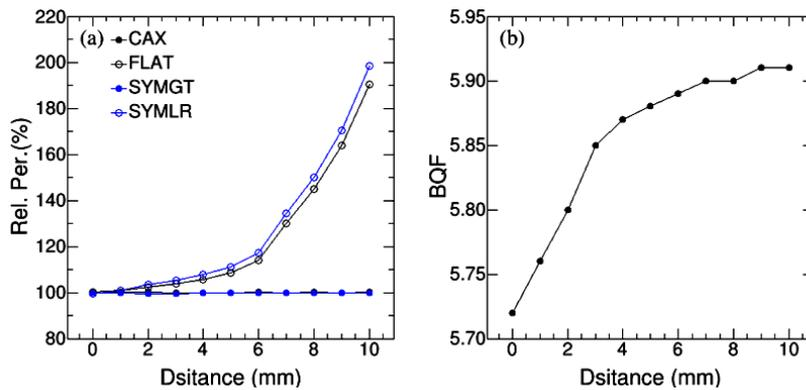
Figure 6. The output of PTW QUICKCHECKweblin in the left-right direction. The abscissa represents the distance from the center. The FLAT, SYMLR and BQF were more sensitive in the left-right direction. The change in this direction exerted little effect on SYMGT and CAX within 1 cm.
