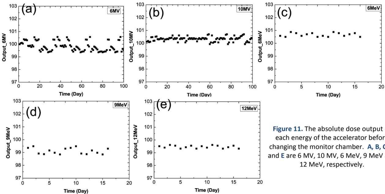
Figure 11. The absolute dose output of each energy of the accelerator before changing the monitor chamber. A, B, C, D and E are 6 MV, 10 MV, 6 MeV, 9 MeV and 12 MeV, respectively.
