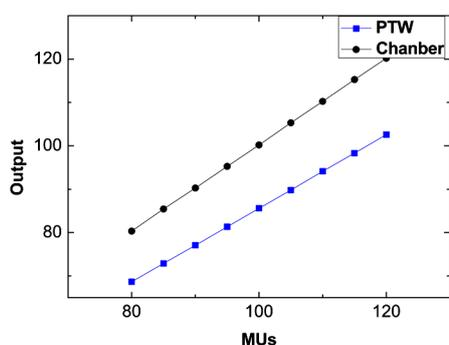
Figure 2. Linearity of the measurements recorded by QUICKCHECK<sup>webline</sup> and the Farmer ionization chamber.
