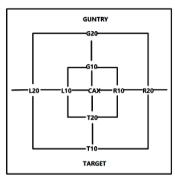
Figure 1. The QUICKCHECK measuring chambers for dose measurements.
