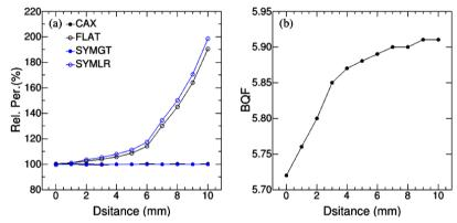
**Figure 6.** The output of PTW QUICKCHECKwebline in the left-right direction. The abscissa represents the distance from the center. The FLAT, SYMLR and BQF were more sensitive in the left-right direction. The change in this direction exerted little effect on SYMGT and CAX within 1 cm.
