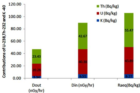
Figure 6. Contributions of <sup>40</sup>K, <sup>238</sup>U and <sup>232</sup>Th to D<sub>out</sub>, D<sub>in</sub> and Ra<sub>eq</sub>.
