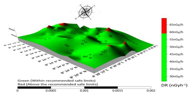
Figure 5. IsoDose-rate map of the laterite mining field.
