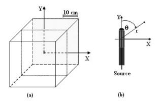
**Figure 3.** Schematic diagram of water phantom and <sup>192</sup>Ir source located in the centre of water cube (a). Representation of the source in a larger size (b).
